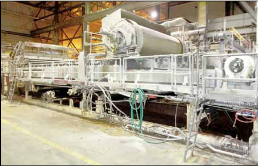
BLACK CLAWSON FOURDRINIER-TYPE PAPER MACHINE #4 – PARTIAL VIEW
